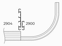
combining wide profile 2904 with 90 degree return 2900-R-W, connected via rail connector 2952.
