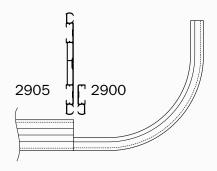
combining wide profile 2905 with 90 degree return 2900-R-W, connected via rail connector 2952.
