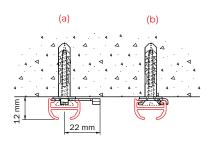
Ceiling mounting with fixing clamp 2650 (including washer), before (a) and after tightening the clamp (b).
