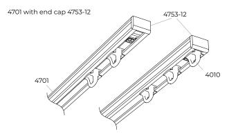
Application of the 4753-12, a product with two functions: only as end cap or as end cap and end stop.
